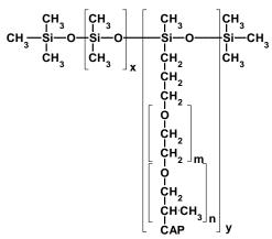
Figure 4: General structure for a silicone surfactant.
