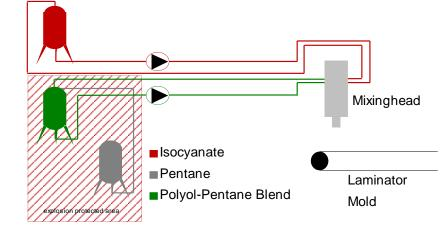
Figure 2: Continuous or discontinuous process for producing pentane blown rigid foam
