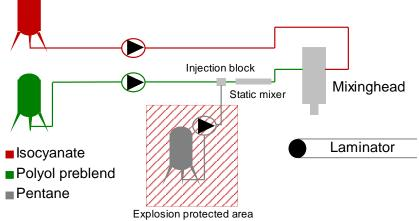
Figure 3: Continuous production of rigid foam panels using pentane as blowing agent
